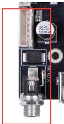
Interface definition as below list, user can apply power board input power supply, port have 6PIN and 2.54mm pin pitch.
