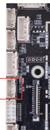
Motherboard provides a 485 serial port which can support mainstream serial ports devices. The voltage for 485 serial ports is 3.3V, if device connected request higher voltage, there must be an isolate circuit or level-shift circuit, otherwise motherboard and device might get burnout.
