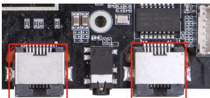
Motherboard provides two connectors, a 100M port and a 1000M port.
