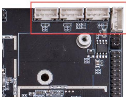
Motherboard provides a USB3.0 standard port and a USB3.0 standard port, four internal USB2.0 ports for peripheral device expansion, USB default mode is HOST, power current must less than 500mA.
