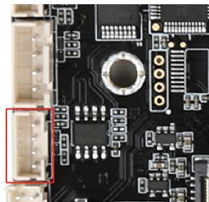
Motherboard provides a 485 serial port which can support mainstream serial ports devices. The voltage for 485 serial ports is 3.3V, if device connected request higher voltage, there must be an isolate circuit or level-shift circuit, otherwise motherboard and device might get burnout.
