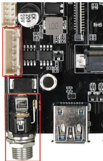
Interface definition as below list, user can apply power board input power supply, port have 6PIN and 2.54mm pin pitch.
