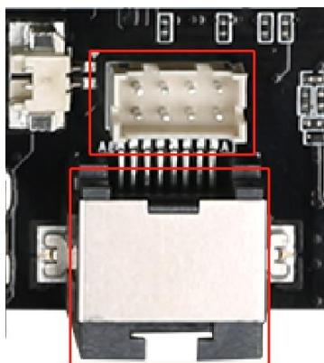
Motherboard supports 1000M Ethernet port, there are two net ports(RJ45 and 8Pin interface), but user can only choose one connector, two ports can't work together.
