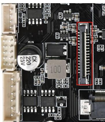
Motherboard can supports MIPI cameras with maximum 1300W pixels, the electrical definition as below:
